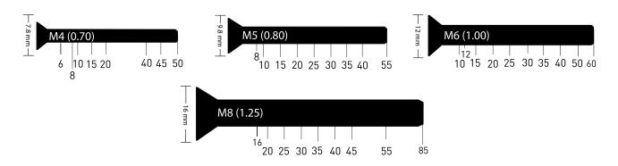
**Dome Head/Fairing Bolts** (Available in Aluminium | Stainless Steel | Titanium ) \*Please Note: Not all combinations of thread length, thread diameter, and thread pitch are available in every material\*
