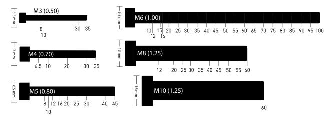
Countersunk Bolts (Available in Aluminium | Stainless Steel | Titanium ) \*Please Note: Not all combinations of thread length, thread diameter, and thread pitch are available in every material\*
