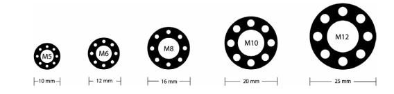
Countersunk Bodywork Washers (Available in Aluminium | Stainless Steel | Titanium ) \*Please Note: Not all combinations of thread length, thread diameter, and thread pitch are available in every material\*
